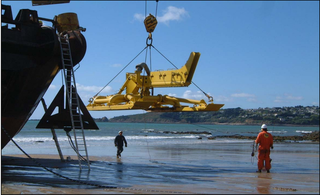
Figure 2-15. Example of Water Jet Trenching Device
